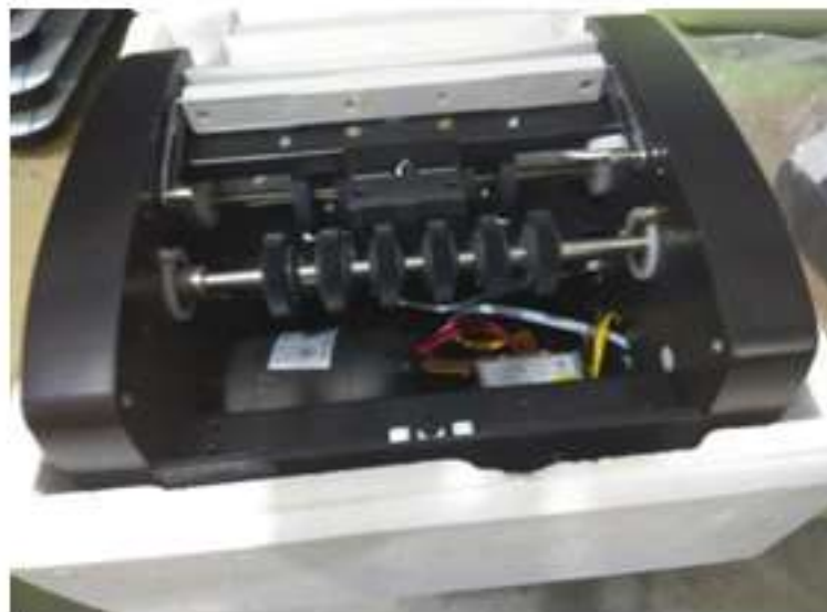
Fig1-The Shaft to be assembled in currency counting machine.
